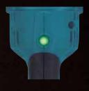
Solid Green indicates that current can be applied to the circuit. (GA9050R / GA7050R)
